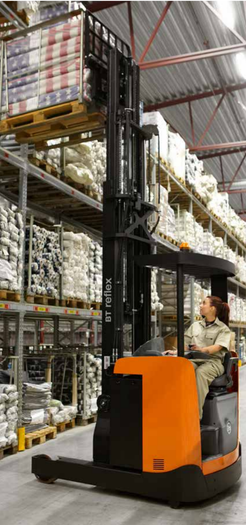
The BT Reflex B-series' controls are easy to use, making the trucks ideal for operators who carry out many other tasks during a shift. For example, the automatic parking brake and tilting forks both contribute to safety and productivity.
